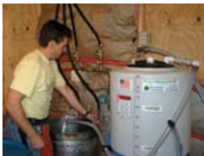
Dave collects used fry oil from restaurants and processes it in a BIODIESEL REFINER to make fuel for the farm vehicles.
